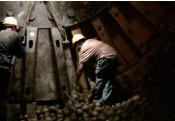
Ø10.37 x 5.19m SAG mill at Dexing Copper with rubber liners after modification
