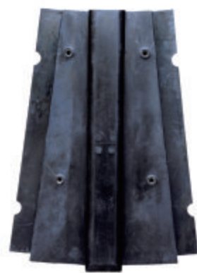
Dashan Concentrator, Dexing Copper, JCC, China: F.E. liners on \varnothing 7.32 \times 10.6 m Ball mill (rubber)
