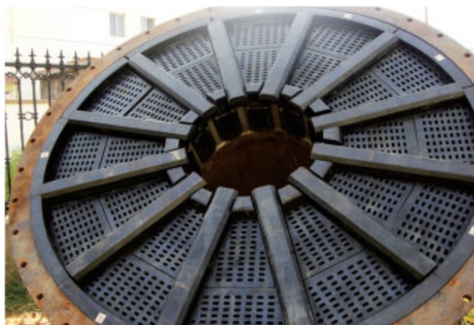
Russia: D.E. grates on \varnothing 3.2 \times 4.5 m ball mill (rubber)
